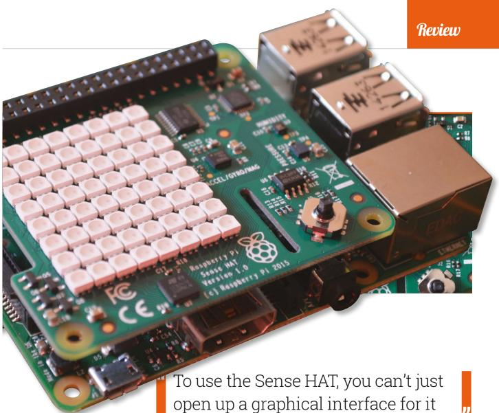
with a trio of positional sensors which include an accelerometer. a gyroscope, and a magnetometer. They're all pretty accurate and able to sense a wide range in their respective fields, with the outputs instantly modified to be readable with the Sense HAT library.
