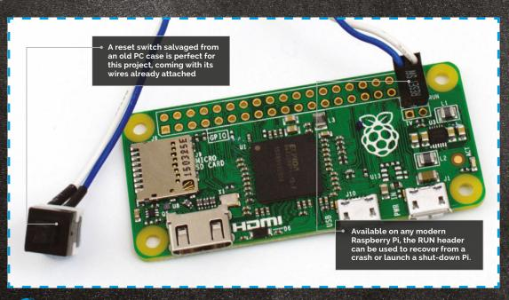
he Pi Zero's diminutive size, low cost, and tiny power requirements mean it's a great fit for embedded projects. There's only one problem: how to quickly get things back up and running if your code hits an infinite loop or otherwise crashes the Pi Zero, especially in projects where the Pi Zero is locked away from prying hands and powered by a hard to interrupt internal battery.
