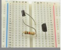
breadboard. The resistor can be connected either way around. To prevent accidental shorts between the resistor and diode leads, it is a good idea to shorten one or both of the leads.
