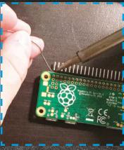
When you're done, save the file and shut down the Pi so that you can solder the headers, add the Pi Traffic Light, and attach it where you need it.
