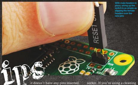
it doesn't have any pins inserted. While it's possible to solder a switch directly to the header, doing so will block the GPIO and TV headers; it's better to solder male pins into the header and run wires to the reset switch.
