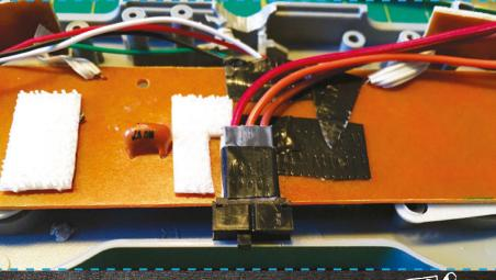
in the cables to ultimately connect the other end to your Pi Zero. To keep things really simple, we're going to connect a slimline mini HDMI-to-HDMI cable to the Zero inside the controller. With our controller, it's actually really easy just to line up the HDMI cable with the USB cable exit on the controller itself, but you'll need to use a craft knife to carve a larger opening and carefully strip back the housing of the mini HDMI connector to get it to fit snugly.
