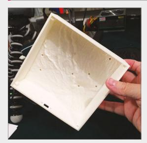
**Above** The 3D printed model with scaffolding removed **Below** A breadboard prototype was used to test the system
