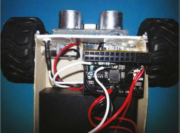
repurposed the parts of a CamJam EduKit 3 to build it. "It's built from a large matchbox, two tiny geared motors, plus wheels, and the rest (motor drivers, sensors, and battery box) is mostly from a CamJam EduKit 3. There's also a 5V regulator so that it can use the motor battery to power the Pi."
