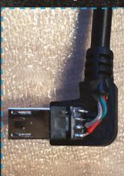
the future, we've decided to take the less invasive route of ripping up a separate micro USB cable and soldering that to the PowerBoost instead.
