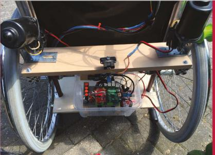
**Above** A windscreen wiper motor is connected to a small 3D-printed wheel. This small wheel drives the main wheelchair wheels
