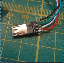
header facing up and towards you, the colour-coded USB cables you snipped off earlier are soldered from left to right as black, green, white, and then red. With the micro USB connector soldered, all you need to do now is preconfigure your Pi Zero with RetroPie and you're ready to go!
