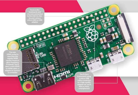
The Pi Zero board uses the same micro USB power input as other Raspberry Pi devices, and you can you to turn the Pi Zero into a super low-cost camera for taking photos and recording videos.
