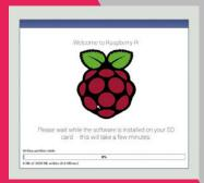
then you download the operating system as an image file, a large file ending in '.img'. This file is then copied bit by bit as an exact replica to the micro SD card.
